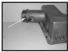
Step 6 Remove the MAFS from the factory intake tube
